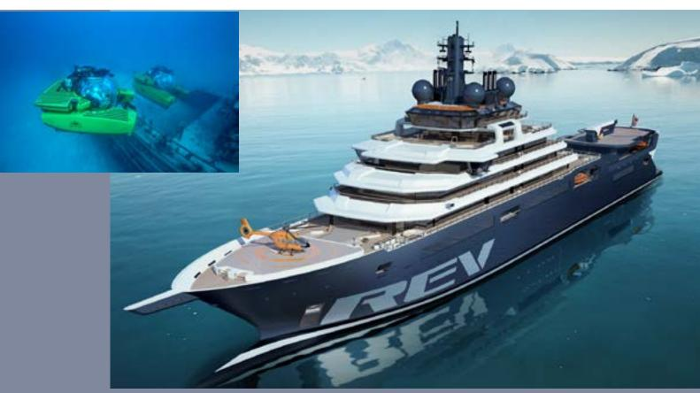
Top – Triton: a three-person ocean research vessel with a diving depth of 2300m that will be used by researchers on REV I. Bottom – Rendering of REV I, the largest, most advanced marine research platform in the world, currently being built in Norway, will help the world to better understand our oceans and what is happening to our marine resources. Photos: REV Ocean
